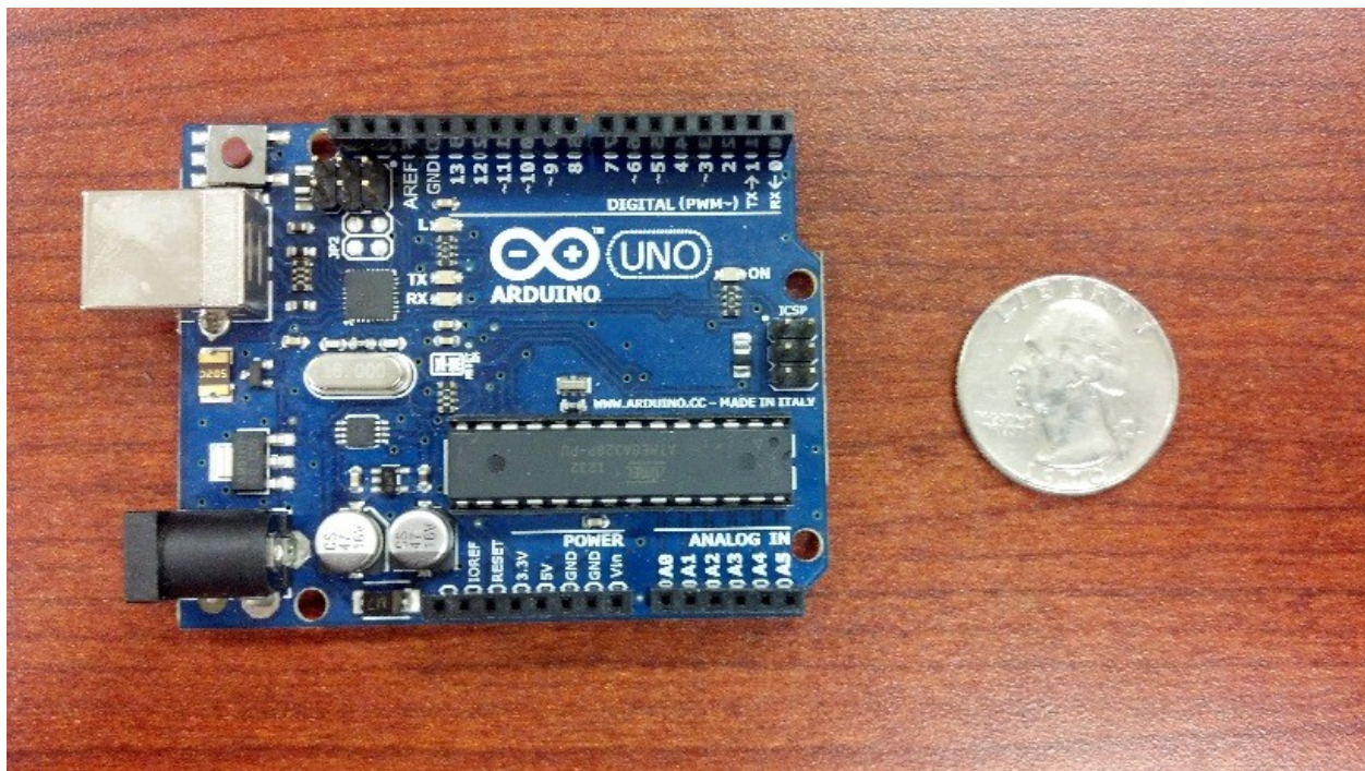
Pictured: An Arduino Uno next to a quarter for a scale reference
